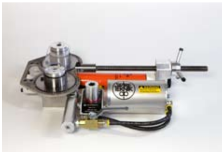
An example of A200 fitted with Hydraulic pump unit PHU1.
